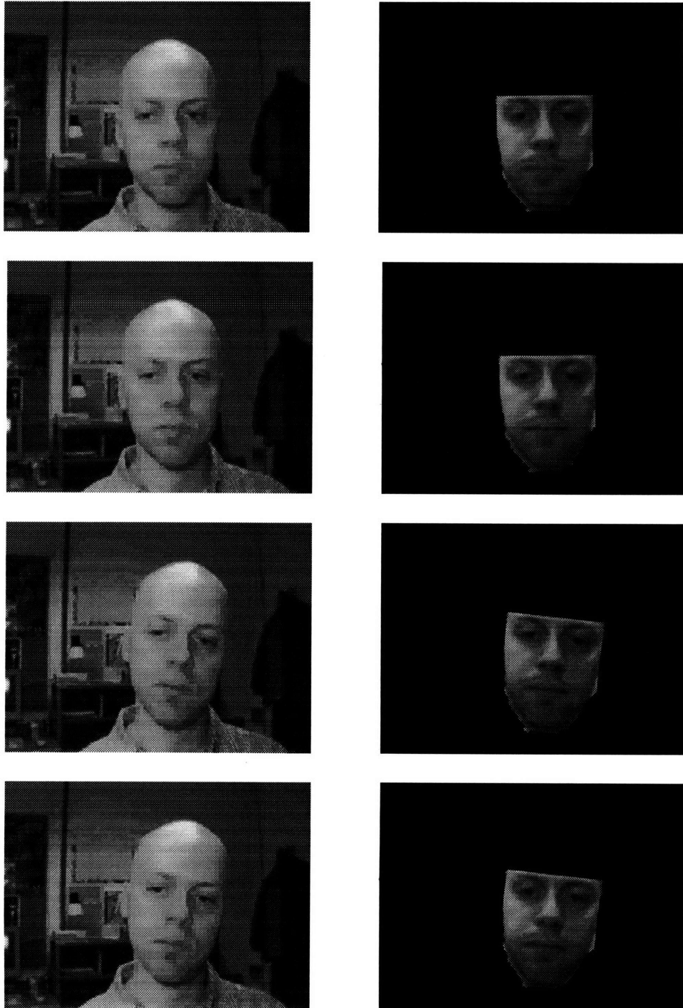
Figure 3-29: A novel sequence with affine movement in which the head rotates, juxtaposed along with the synthesized sequence.
