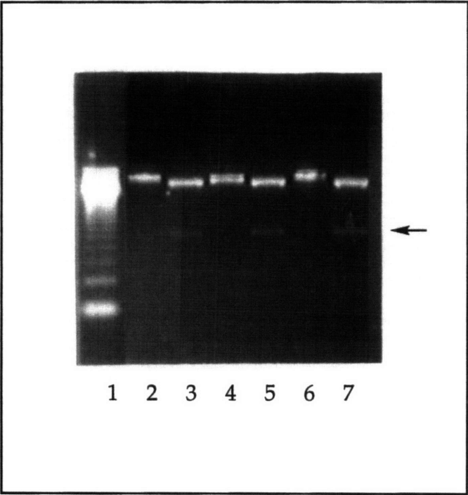
Figure 4.13 DNA gel electrophoresis of the restriction digest of plasmids containing the truncated apoE sequence isolated from three colonies (colony 1: lanes 2 and 3, colony 2: lanes 4 and 5, and colony 3: lanes 6 and 7). Lanes 2, 4, and 6 show the uncut plasmids, and lanes 3, 5, and 7 show the plasmids with two cuts and a liberated DNA fragment. Lane 1 is a 123 DNA base-pair ladder standard. The arrow indicates the excised 507 base-pair fragment.
