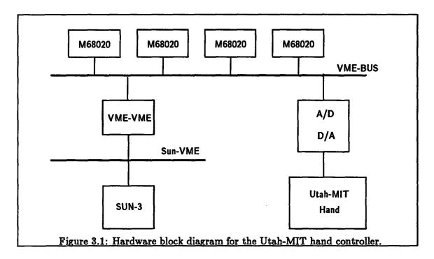
In this document, we do not discuss either the arm control hardware or the analog controller hardware designed for the Utah-MIT hand. Our emphasis will primarily be on the Motorola 68020 system designed to run control software and the development software that presently runs on the Sun.
