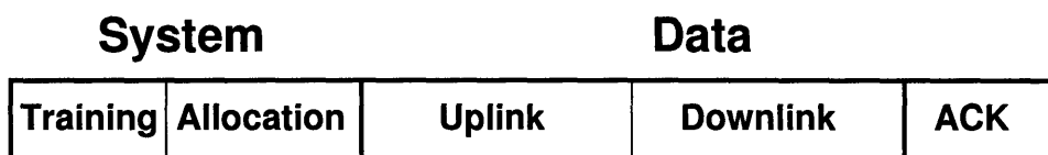
Figure 3-2: The five phases of a communications frame.
