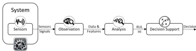
Figure 2. Block Diagram of classic PHM
