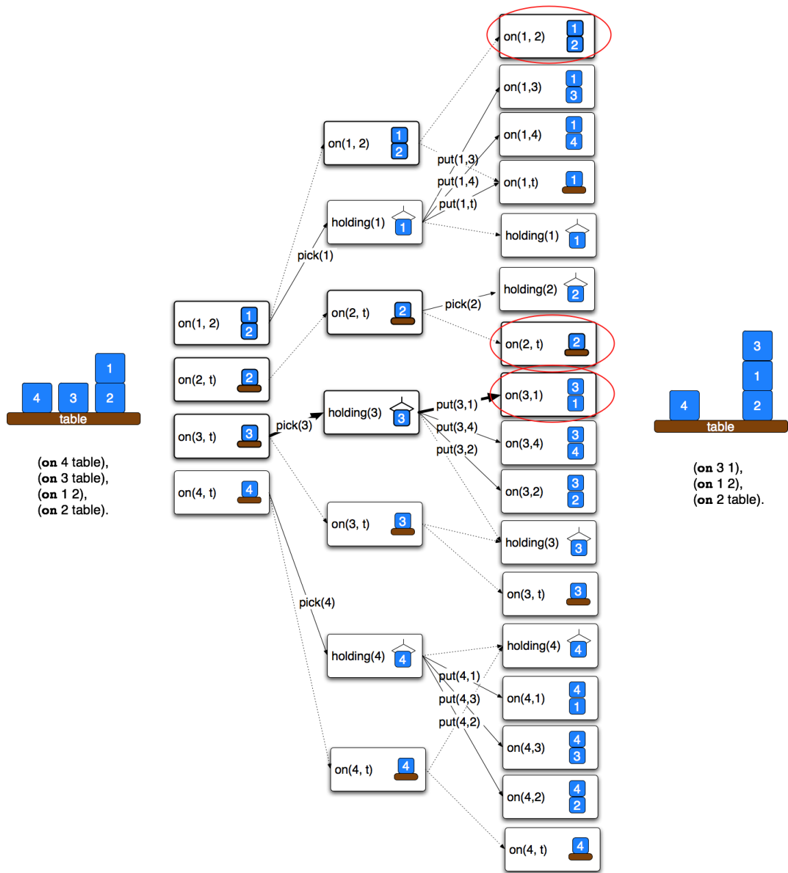
Figure 3-2: An illustration of the Graphplan algorithm finding a solution for a block-stacking task given the initial state at left, and the goal condition at right. Maintenance actions are shown with dotted lines. For simplicity, the mutual-exclusivity constraints are not shown.
