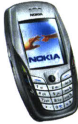
Figure 2. The Nokia 6600, a Symbian Series 60 Phone. This phone comes with 6 MB of internal memory and a 32MB MMC flash memory card. Custom applications can be loaded onto the phone from the GRPS data network, Bluetooth, memory card, or the infrared port.
