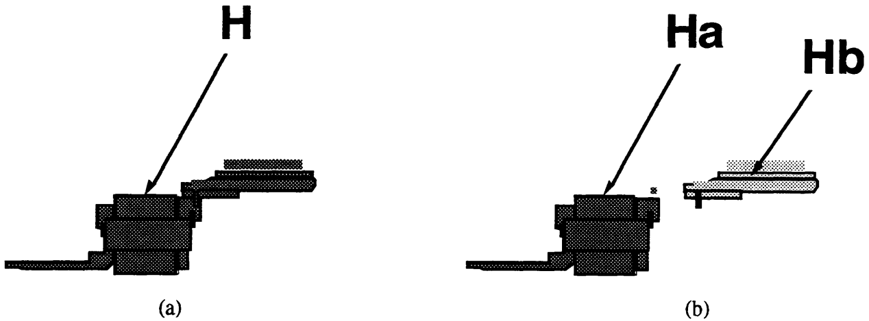
Figure 4-3: (a) original subassembly H; (b) broken down into subassemblies Ha and Hb
