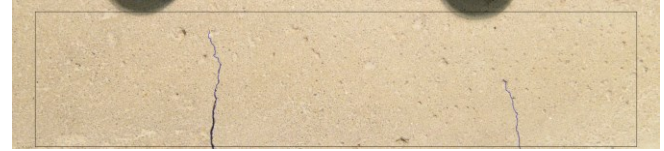
Figure 7 First two cracks formed on the concrete surface (rough surface)
