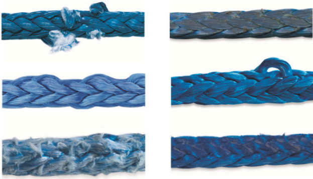
Figure 5. Different kinds of rope damages. Cut strands (top left), compression damage (top right), inconsistent diameter (middle left) and pulled strands (middle right), heavy abrasion (bottom left) and melted fibers (bottom right). Reproduced with permission from Samson Rope Technologies.
