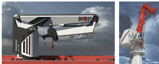
Figure 1. Fiber rope cranes by National Oilwell Varco (left) and MacGregor (right). Reproduced with permissions.
