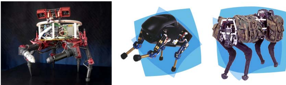
Figure 5-4: Examples of Legged Robots from Left to Right: LEMUR, LittleDog, and BigDog [Volpe 07] [BDI 07]
