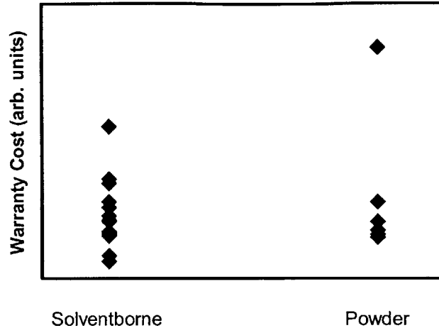
Figure 3.1. Normalized warranty cost comparison for vehicles coated with powder- and solvent-based primer surfacer.
