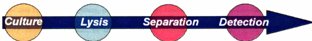
Figure 1. 2: Schematics of an integrated \mu TAS. The system consists of several integrated sample preparation modules, such as cell culture, cell lysis, protein and organelle separation, followed by a detection module located downstream of the processing cascade. The arrow represents the order in the process. Even though the process described here is linear, \mu TAS are not limited to linear systems and allow the parallelization of assays for higher throughput or more complex functions.
