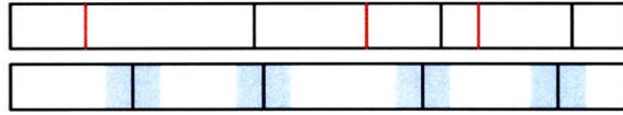
Figure 3-6: An example for measuring segmentation performance (above: detected transitions; below: relevant transitions).
