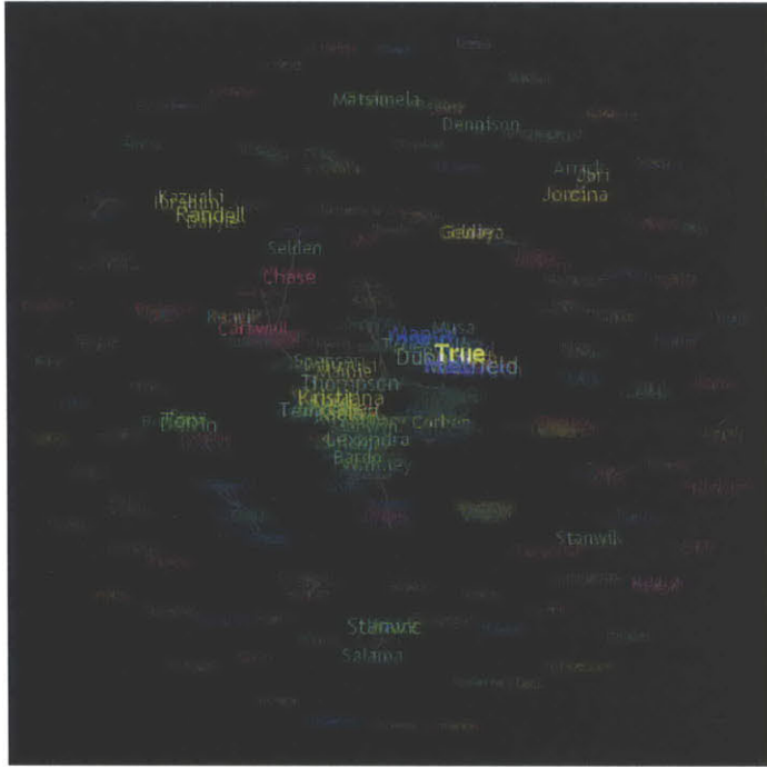
Figure 7-1. This image is derived using our example data provided by Drew. In the image, we see all of Drew's nodes in a position where they've reached a settled layout. The result resembles a galaxy, with various solar systems. Due to the initial random layout and the general centrifugal gravity, this algorithm frequently pulls the most highly connected clusters towards the center.
