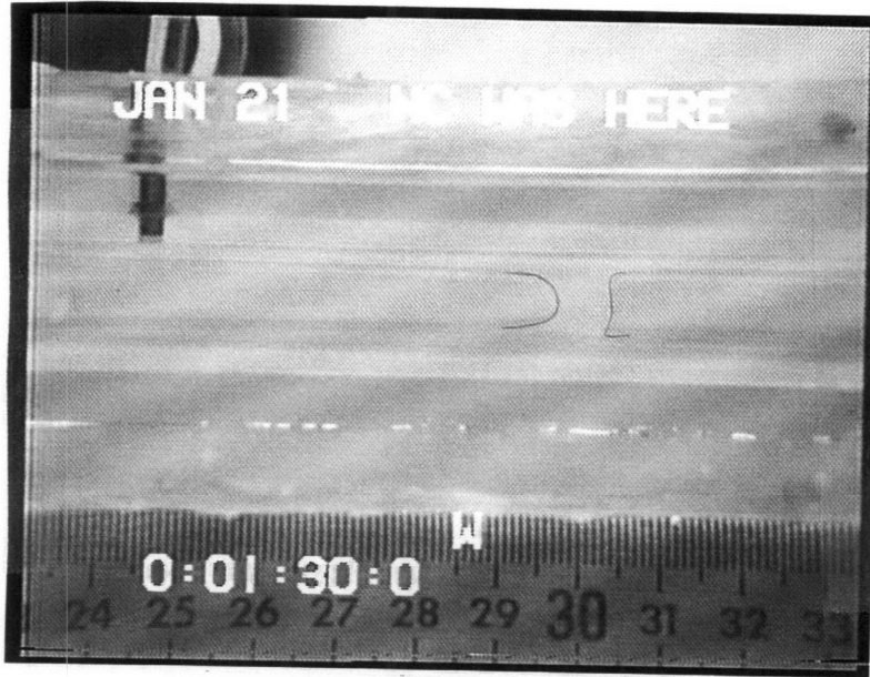
Figure 11. Bullet Shape of Trailing Meniscus (trailing meniscus radius is small, capillary pressure is high)
