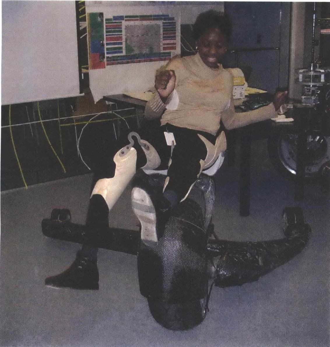
Figure II-10: testing of the humanseat Mk1 mounted on the Mini Athlete. The subject – who does not ski – spontaneously started making skiing and bicycling movements showing visible enjoyment after a short period of familiarization with the seat.
