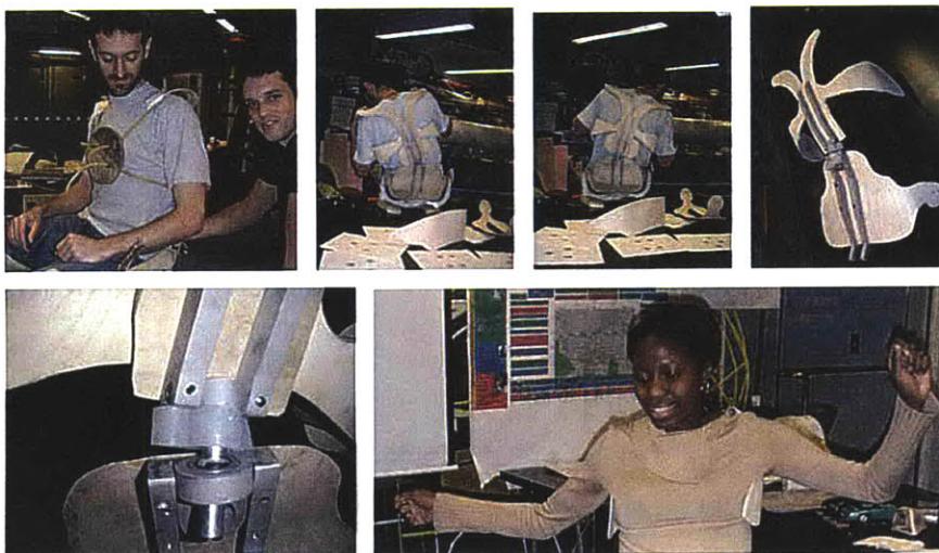
Figure II-23: Development of the upper back support. Unless there needed to be a provision for sudden deceleration, there was no ergonomic reason to have shoulder straps or frontal chest support. A telescoping ball joint with a silicone bushing and a metal stopper provided all the degrees of freedom, damping, and the hardstops needed. Lateral chest support felt comfortable.
