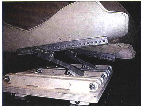
Figure II-27: Movement apparatus using parametric assembly of flextures. Flextures were installed in a manner that the preset angle to the base rail can be varied. The preset angle to the plywood seat pieces can also be varied, as can the longitudinal attachment point. Flextures allow movement in all directions, note movement pattern depending on load. Flextures longitudinally split in the middle with a gap of ca. 1mm were employed at a later stage for better torsional deformation (bottom right panel shows torsional deformation).
