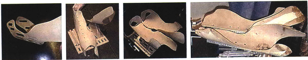
Figure II-30: Evolution of thigh pieces. Original piece for Mk1 seat has lateral support area for hip, but has no support area for buttocks (left). The first pieces for the Mk2 seat have a lower lateral support area for the hips, and the horizontal concave support area is extended back beyond the buttocks (middle left). The second pieces for the Mk2 seat had additional support for the back of the buttocks and were more convex in the medial buttock area (middle right). The final pieces were mildly curved upwards in the back and were lined with suede-like fabric to increase friction. This resulted in an increased range of motion (right panel).
