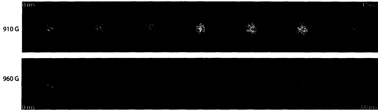
FIG. 1: Superfluid expansion of a strongly interacting rotating Fermi gas. Shown are absorption images for different expansion times on the BCS-side of the Feshbach resonance at 910 G (0.0, 1.0, 2.0, 3.0, 3.5, 4.0, and 4.5 ms) and 960 G (0.0, 0.5, 1.0, 1.5, 2.0, 2.5, and 3 ms), before the magnetic field was ramped to the BEC-side for further expansion. The vortices served as markers for the superfluid parts of the cloud. Superfluidity survived the expansion for several milliseconds and was gradually lost from the low density edges of the cloud towards its center. Compared to 910 G ( a = -7200 a_0 ), superfluidity decayed faster at 960 G ( a = -5000 a_0 ) due to the reduced interaction strength. The total expansion time remained constant [14]. The field of view of each image is 1.2 \text{ mm} \times 1.2 \text{ mm} .
