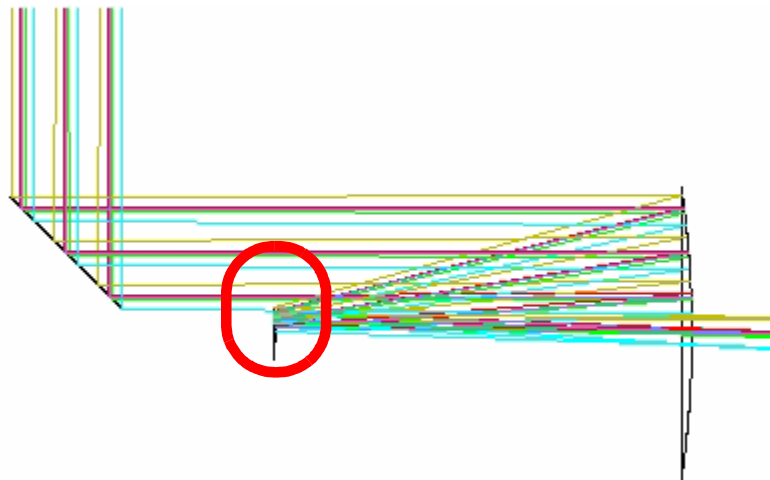
Figure 4.25 Two-mirror (Cassegrain) type beam combiner. The secondary mirror of the beam combining telescope partially blocks the incoming beams.
