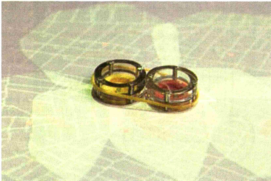
Figure 18: A rubber band used as a mechanical constraint to keep two pucks in close physical proximity.
