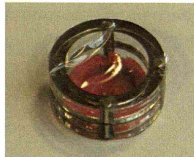
Figure 8: A Pico tag with an LC resonator in the middle and four rare-earth magnets around its circumference
