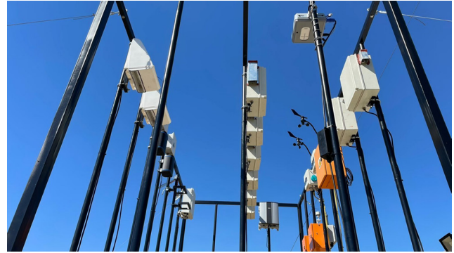
Figure 2: LCS-SA Campaign set-up - various low- and medium cost air quality sensors co-located at the same height on a custom-constructed sensor-stand.
