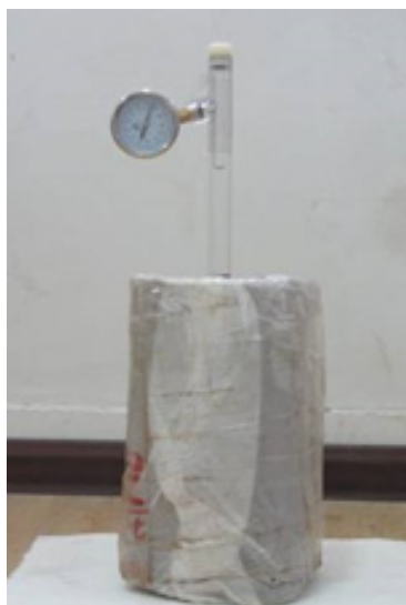
Figure 3. The SWCC test with TEN tension meter
