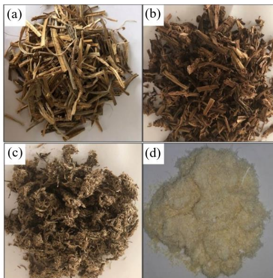
Figure 1 Pictures of (a) raw banana pseudo-stem, (b) after treating with \text{H}_2\text{SO}_4 , (c) after treating with \text{NaOH} , and (d) final product after treating with \text{H}_2\text{O}_2
