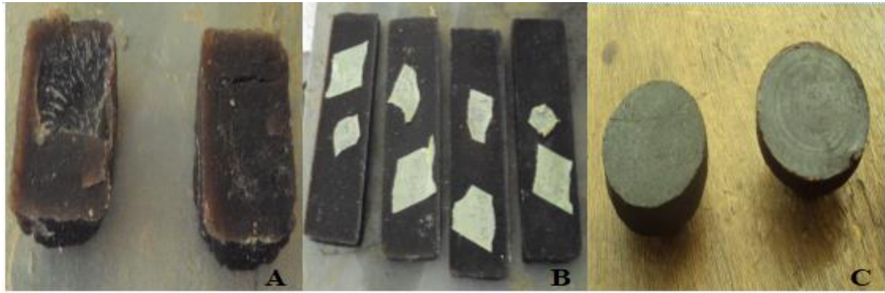
Figure 1 Test samples for (a) compression strength test (b) oil and water absorption test (c) wear test
