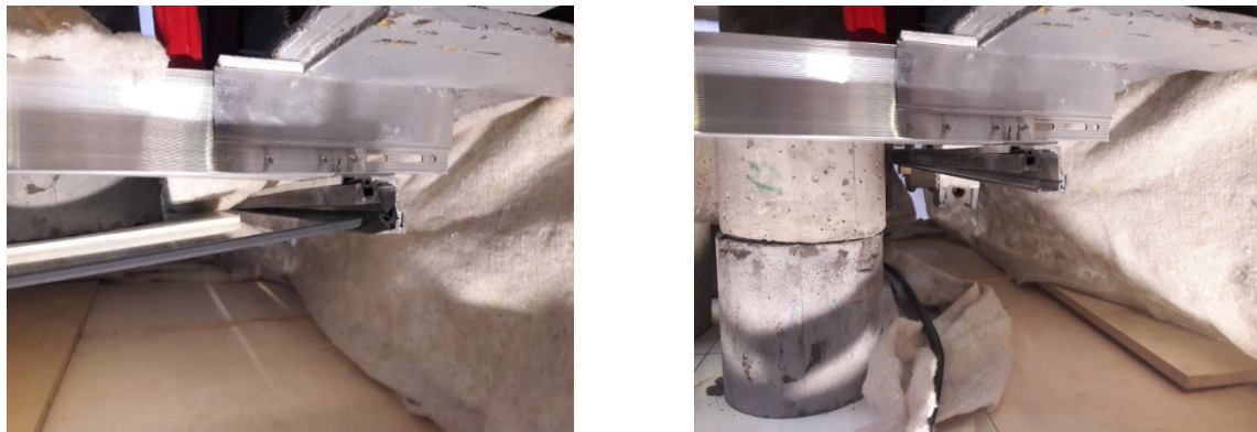
Figure 29. Deformation of sealant (test setup 1).
