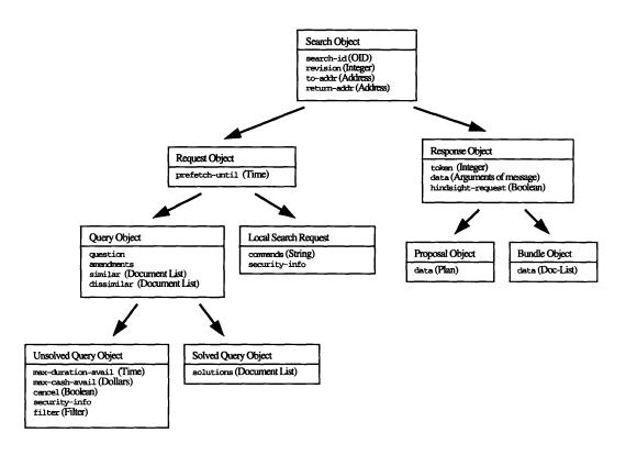
Figure 4-1: The Search object Hierarchy. Arrows indicate the child's inheritance of the parent's fields.
