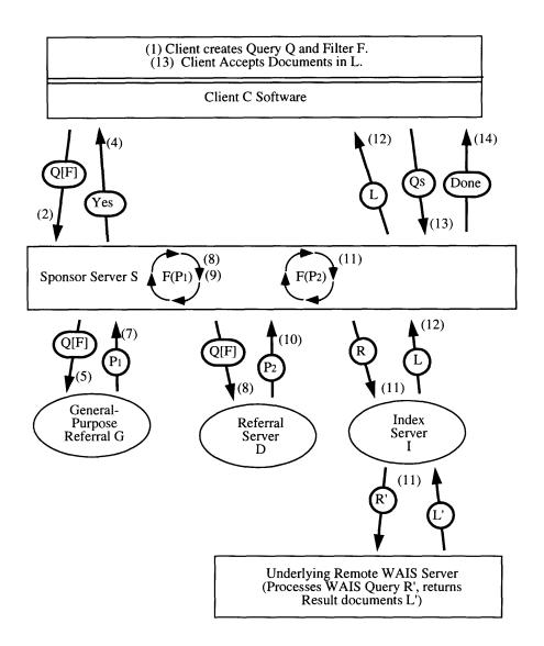
Figure 3-1: A brief example of the meshFind system in action.
