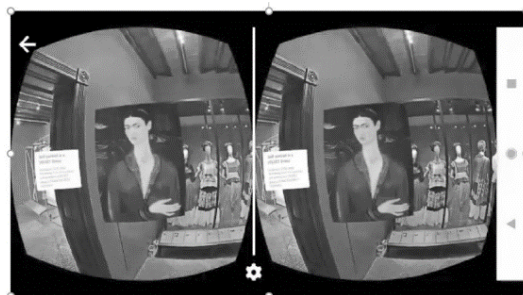
Figure 6. One frame of the scene about Frida's dresses. After clicking on a text icon, the viewer sees one targeted word displayed in context. An image follows the text (here, Frida's first self-portrait). The lenses inside the Google Cardboard™ converge the two images into one, giving it the illusion of three-dimensional space.
