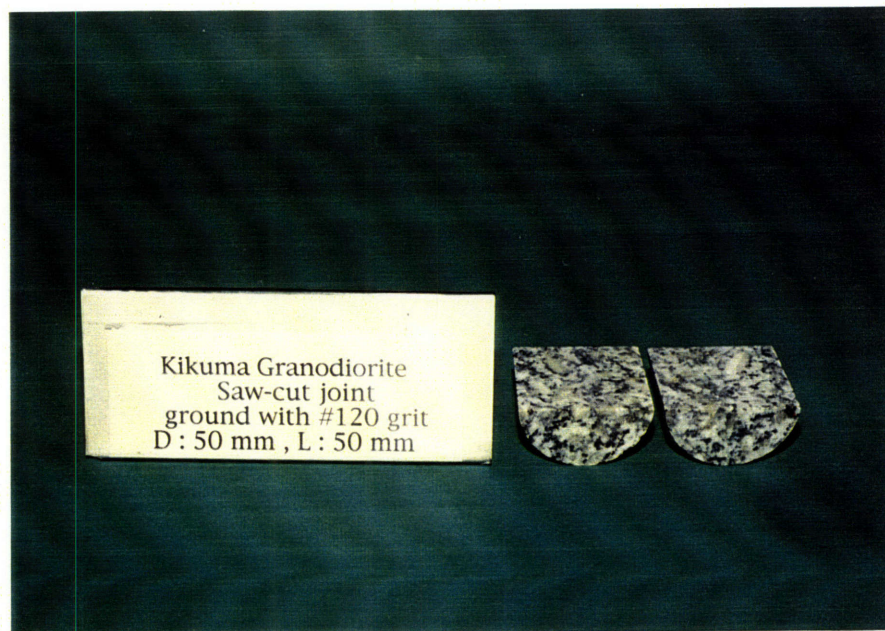
B.3 A photograph of a sawed joint in Kikuma granodiorite (L=5 cm)
