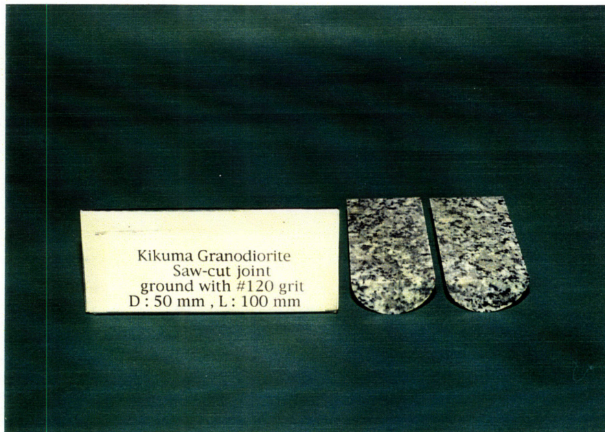
A.3 A photograph of a sawed joint in Kikuma granodiorite (SKGD, L=10 cm)
