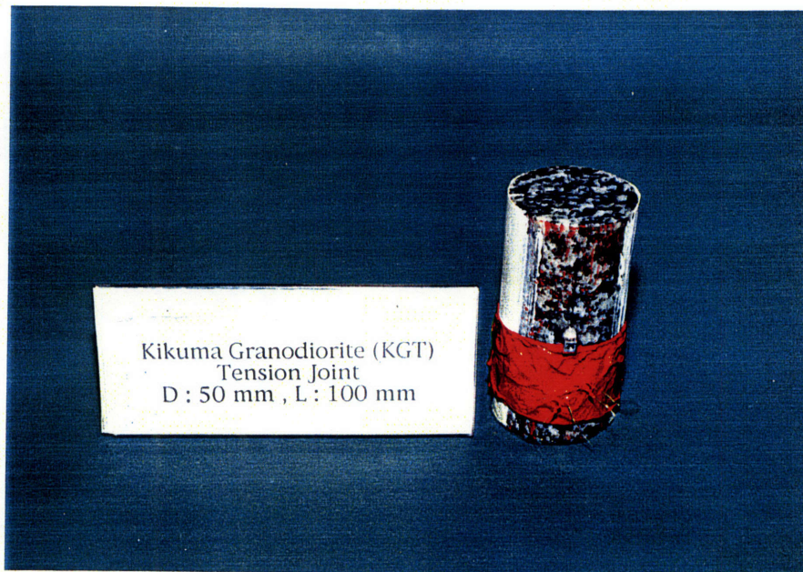
Fig.5.5 Photographs on the procedure for the sample preparation (b) Enclosing the affixed strain gauges with silicon rubber
