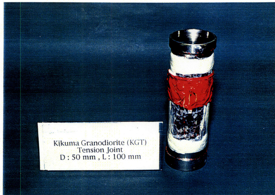
Fig.5.5 Photographs on the procedure for the sample preparation (c) Sealing both ends of a specimen with epoxy
