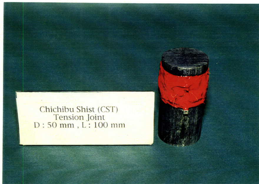
A 5 A photograph of a tension joint in Chichibu schist (TCSH, L=10 cm)
