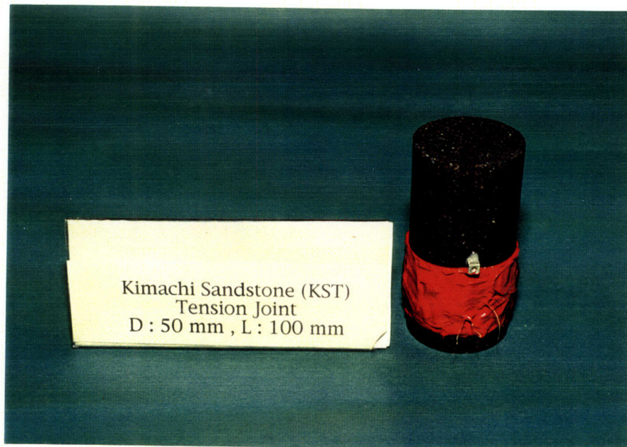
A 6 A photograph of a tension joint in Kikachi sandstone (TKSS, L=10 cm)
