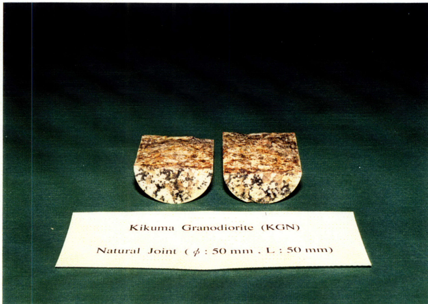
B.1 A photograph of a natural joint in Kikuma granodiorite (L=5 cm)
