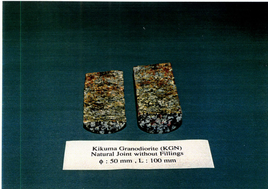
A.1 A photograph of a natural joint in Kikuma granodiorite (NKGD, L=10 cm)
