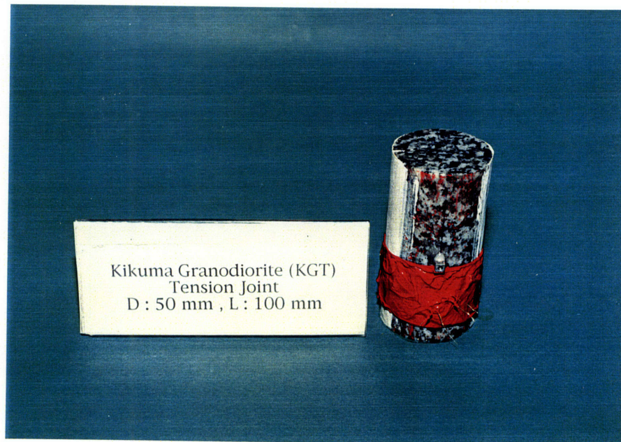
A 2 A photograph of a tension joint in Kikuma granodiorite (TKGD, L=10 cm)
