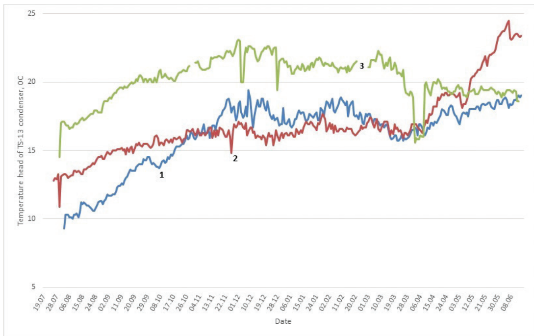
Figure 3. Temperature head change for the TS – 13 condenser: 1 – temperature head in 2016–2017; 2 – temperature head in 2017–2018; 3 – temperature head in 2018–2019
