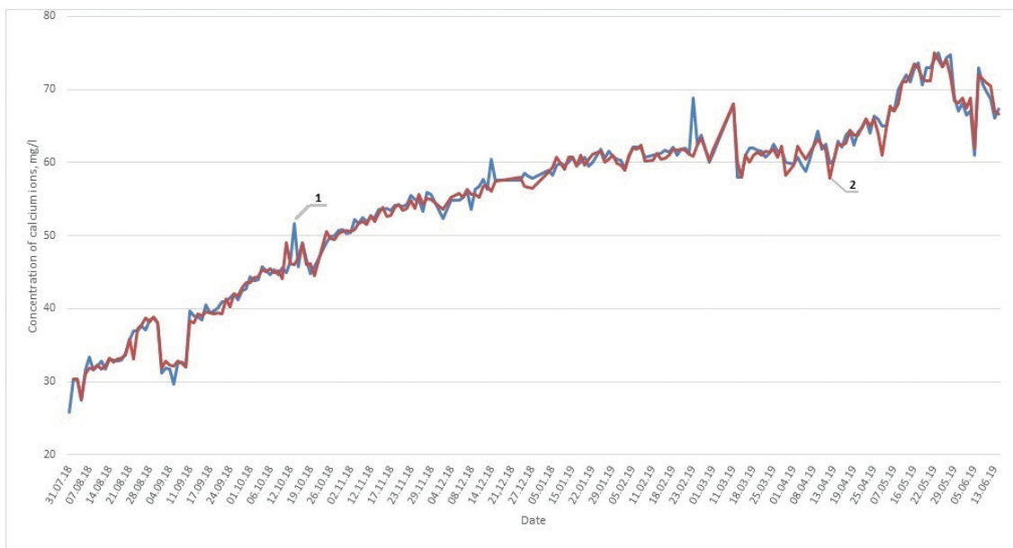
Figure 2. Content of calcium ions in the cooling water at the condenser inlet and outlet: 1 – concentration of calcium ions at the TS-14 condenser inlet; 2 – concentration of calcium ions at the TS-14 condenser outlet
