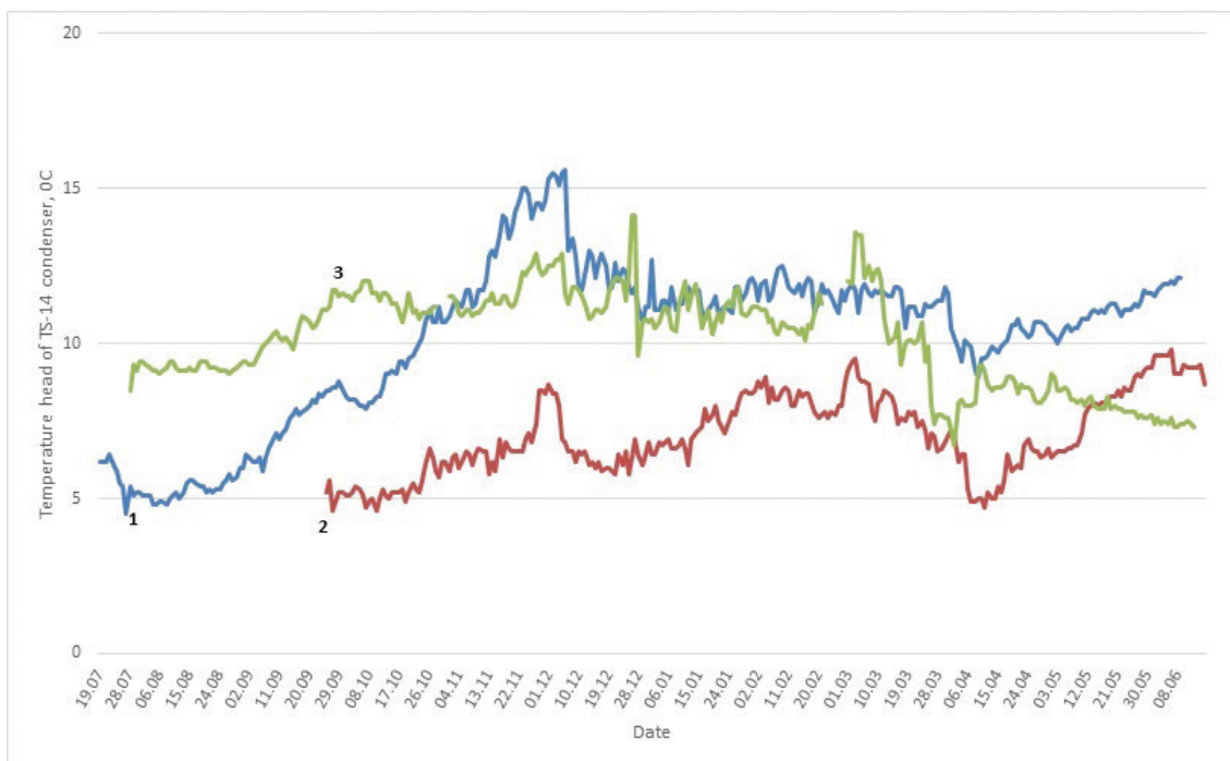
Figure 4. Temperature head change for the TS-14 condenser: 1 – temperature head in 2016–2017; 2 – temperature head in 2017–2018; 3 – temperature head in 2018–2019
