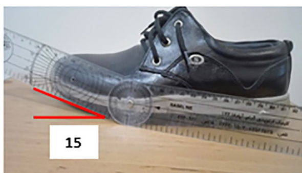
Figure 2: Rocker bottom shoe
