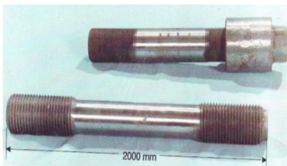
Fig. 2. Fasteners of steel 30Cr2NiMoVN. Length 2000 mm, diameter 120 mm [10]
