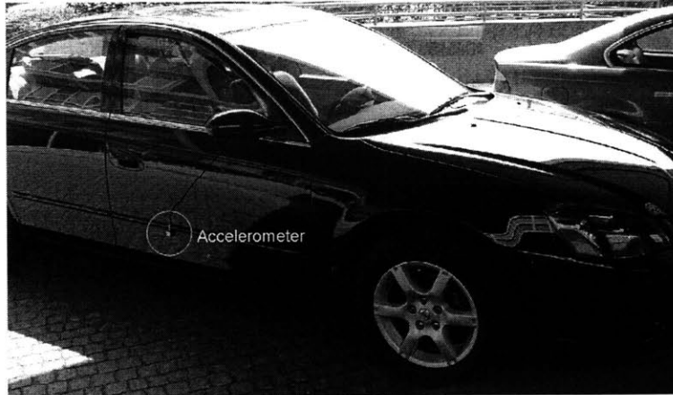
Figure 6-2: Placement of a three-axis accelerometer on a car door to collect vibration data.
