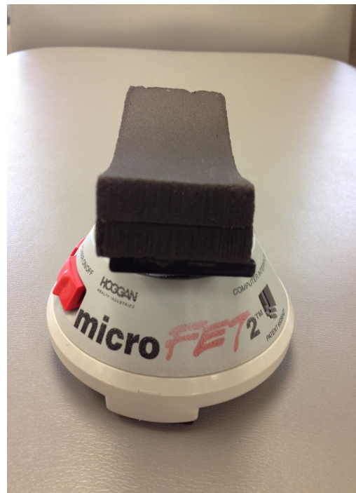
Figure 4: Hand held dynamometer used for strength measures .
