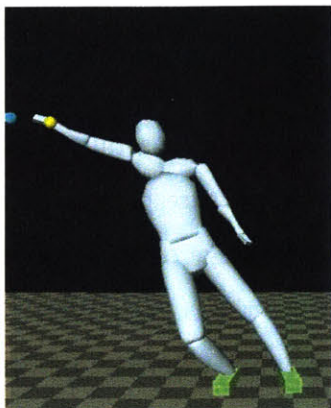
Figure 4-4: This illustration underscores the importance of incorporating ground contact constraints into any control formulation. Ignoring contact dynamics, a character can reach for the object as if his feet were pinned to the ground. With proper contact dynamics and multiobjective control, the character strikes a compromise between reaching and not falling as seen in Figure 4-3.
