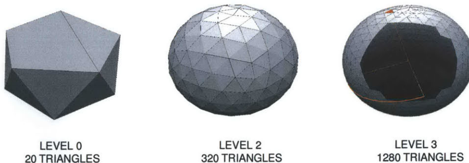
Figure 3-6: Sphere tessellation by icosahedron subdivision. Edges are sorted according to the index of the facet pointed to by the normal vector to the edge (in red).
