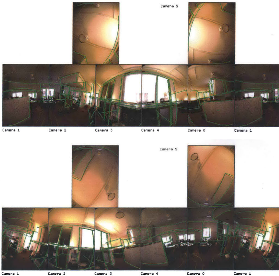
Figure 8-15: HAND-HELD dataset; 3D model re-projected on the video.
