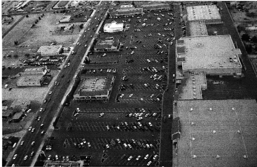
Figure 1-5: Latter 20th century arterial streets, often begin as a rural highway (top) and develop with ample setbacks, parking and big box retail (bottom).
