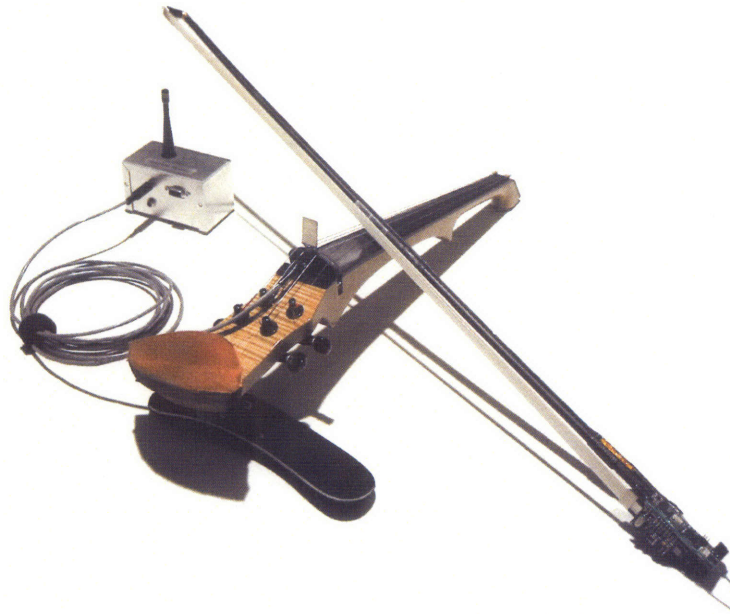
Figure 2.1: The Hyperbow sensing system that was developed for the Toy Symphony project was installed on a Jensen electric violin and a CodaBow® Conservatory™ carbon fiber violin bow. The system was optimized to be lightweight and compact and relied on minimal external electronics.
