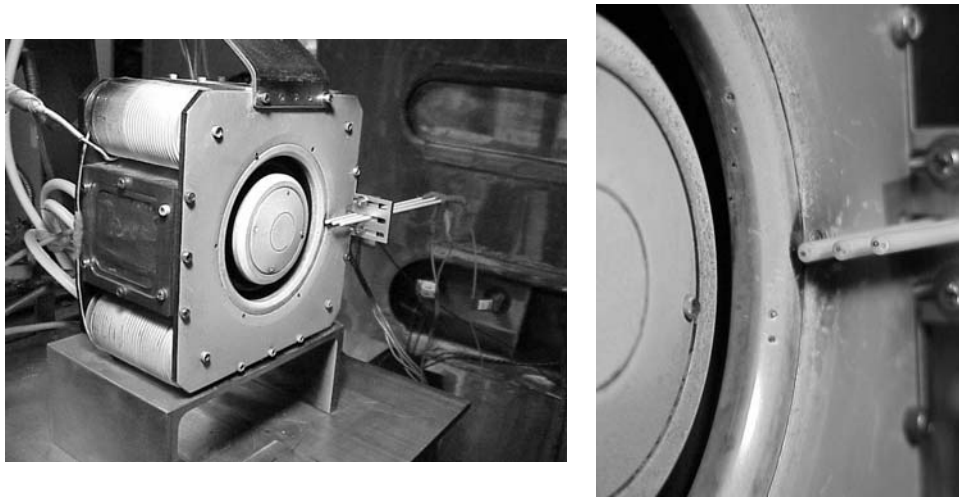
Figure 3.15 Photographs of the low voltage test setup. Note that there is an extra hole near the chamfer probe that was not used.
