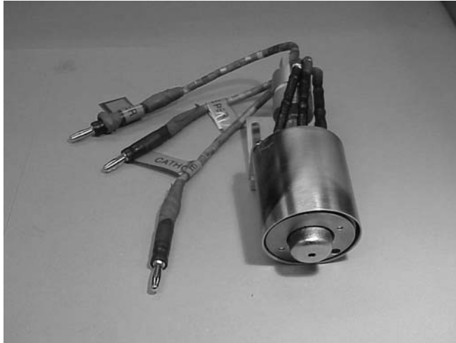
Figure 2.3 The HCN-252 Hollow Cathode Neutralizer built by Ion Tech, Inc. is used with the BHT-1000.
