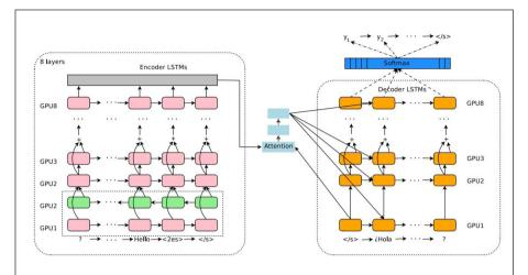
Figure 14. The model architecture of the multilingual GNMT system (Melvin Johnson et al., 2016).
