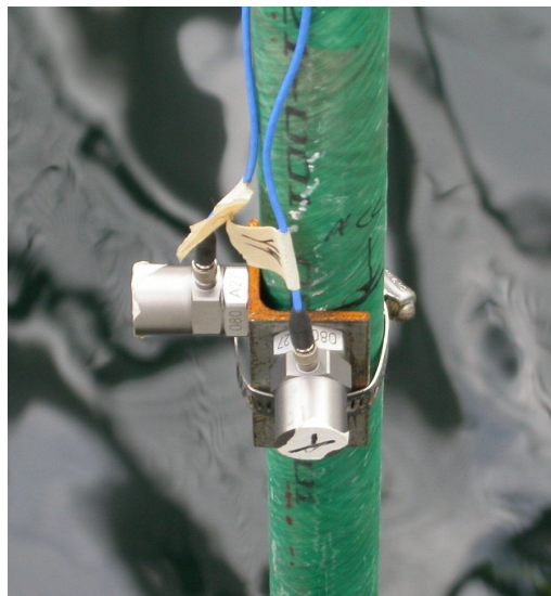
Figure 86 – Accelerometers used in the mechanical shake-down test and the impact testing
