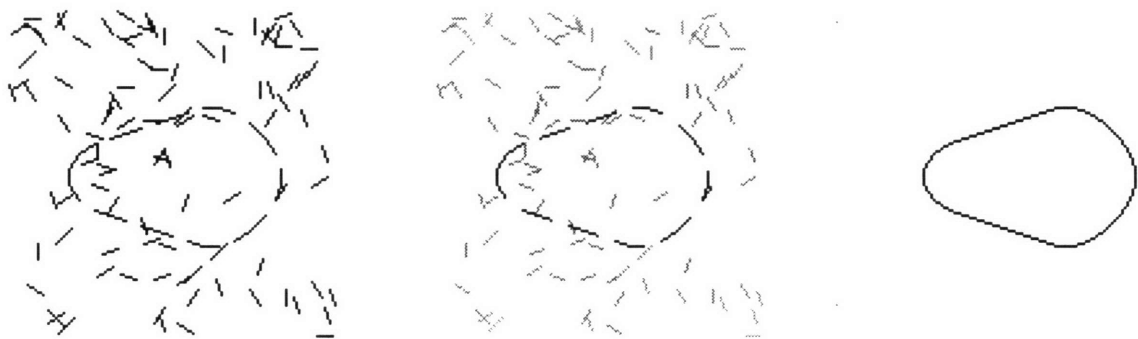
Figure 3-8: Left: smooth, fragmented shaped on a noisy background. Middle: shortest-paths saliency map. Right: the most salient curve ( S = 0.5445 ).
