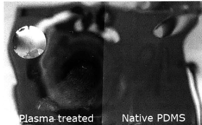
Figure 4.15. Results of E-beam evaporated silver mirrors on (left) an air plasma treated PDMS surface and (right) a native PDMS surface. The camera reflection from the native PDMS surface is much more diffuse than the camera reflection from the plasma treated PDMS surface.
