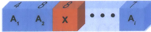
Figure 2-4: One gene mutated from a value of A_3 to a new value of X . The new value X comes from the same set of possible values of this particular gene which in this case is from the 8 possible integer values.
