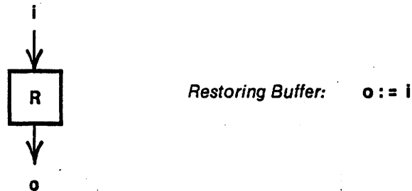
Figure 2-4: Restoring Buffer Schematic
