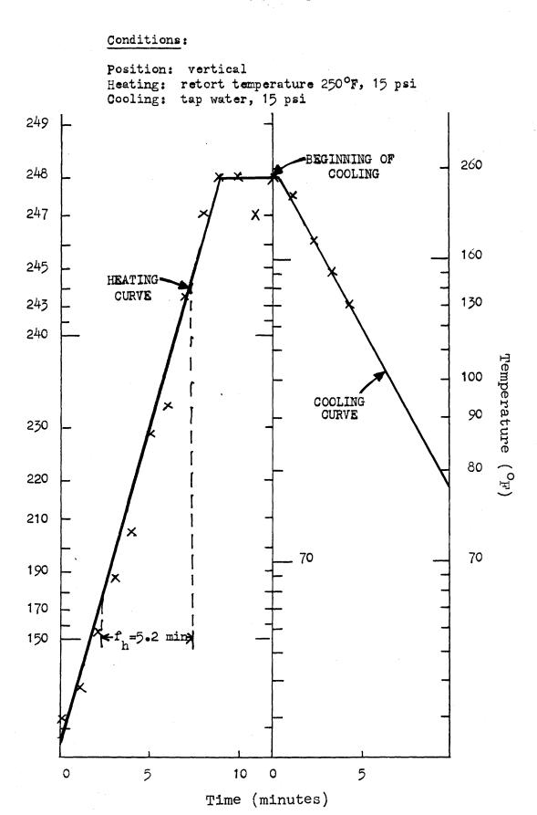
Figure 5 Heat Penetration Curve For Carrot Slices In Chicken Broth
