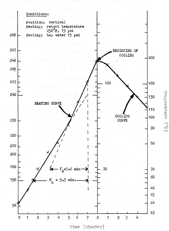
Figure 3 Heat Penetration Curve For Chicken Broth At Slowest Heating Point
