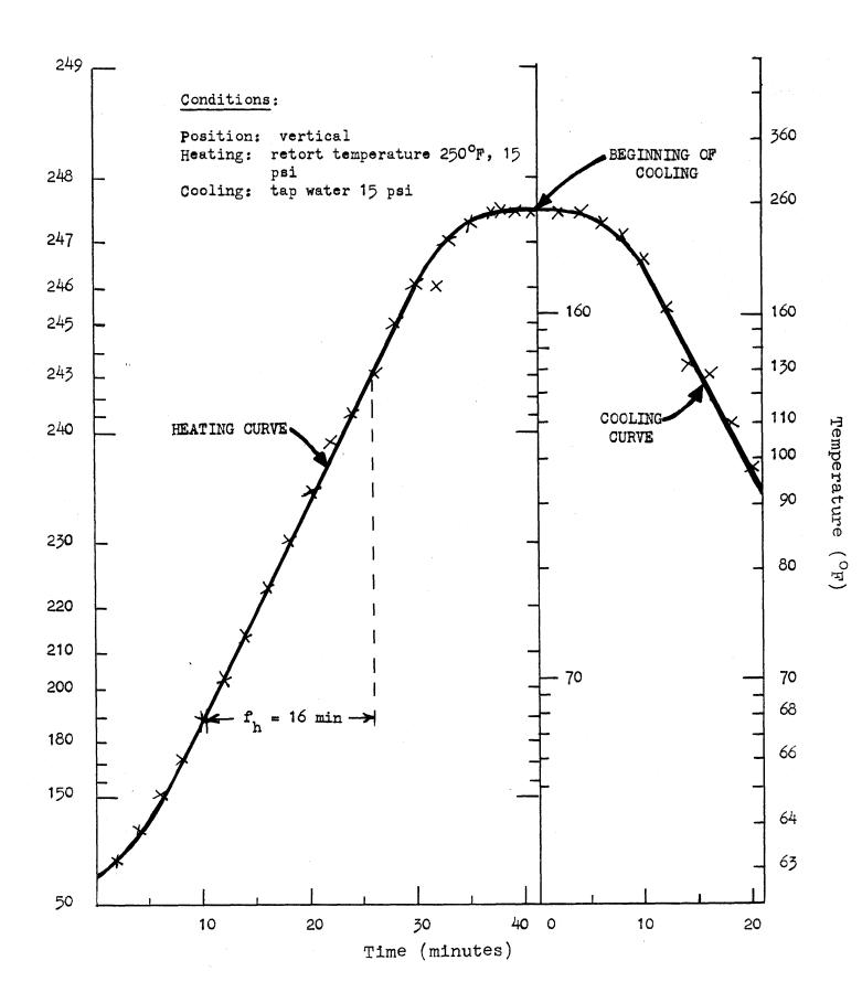
tical positions (actual experimental data from package # 2, Run GB V-VI), having the average value for time required to reach  $240^{\circ}F$  and  $245^{\circ}F$  and to traverse one log cycle of temperature is presented in Figure 1.
