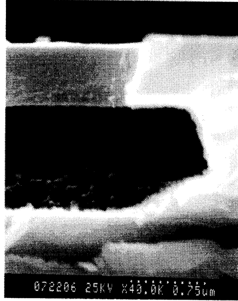
Figure B.2: Morphology of the etched surfaces. The roughness on the surface of the sacrificial layer under the beam is visible.
