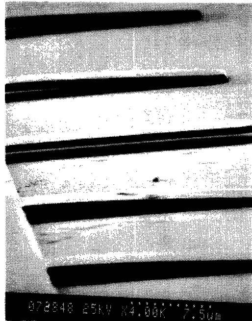
Figure 4.14: SEM photograph of GaAs/InGaP cantilever structures. The structures are 20 \mu\text{m} long and the only free-standing structure is 4 \mu\text{m} wide.
