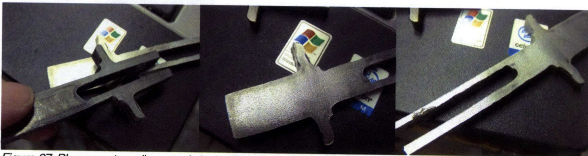
Figure 27: Plasma cut medium steel shaft. Plasma cutting was unable to give straight perpendicular cuts necessary for this design.
