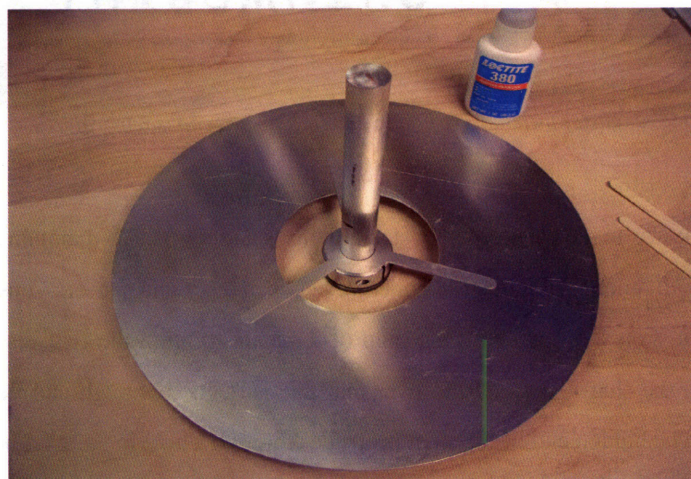
Figure 19: Assembling the disc pack onto the shaft
