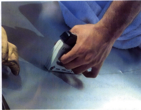
Figure 7: Stapling aluminum flashing to shaping ribs to form parabolic reflector trough.
