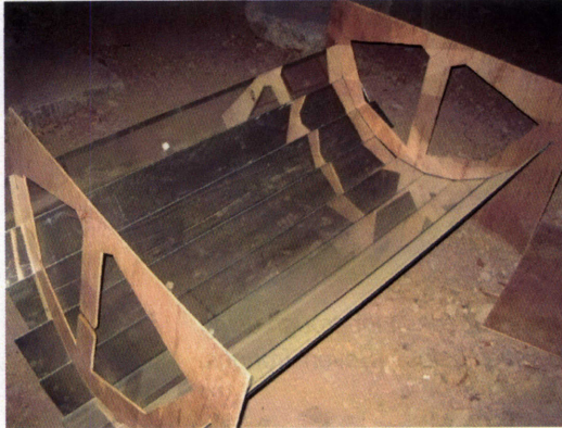
Figure 8: One night's dirt accumulation on trough. (Pabal, India)
