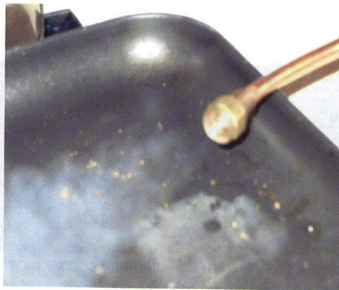
Figure 13: A well formed jet of steam from the pressure cooker boiler.
