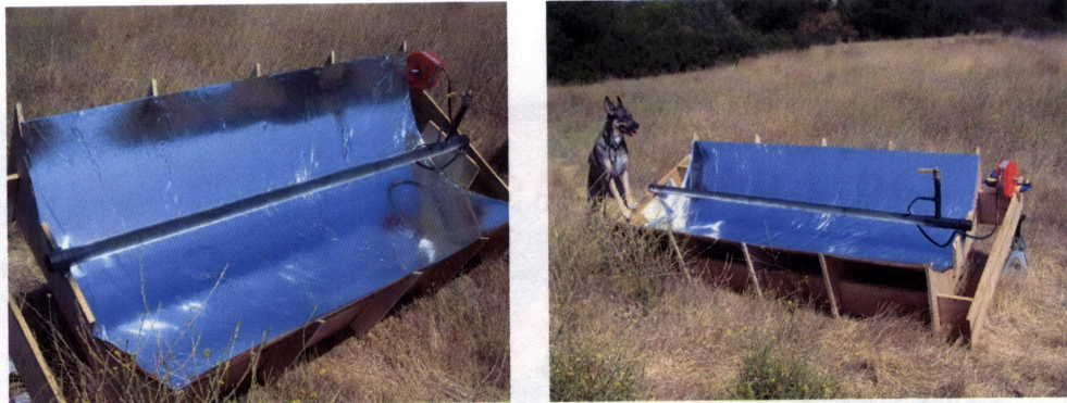
Figure 3: Integrated solar collector, boiler, and turbine. (Calero State Park, California)
