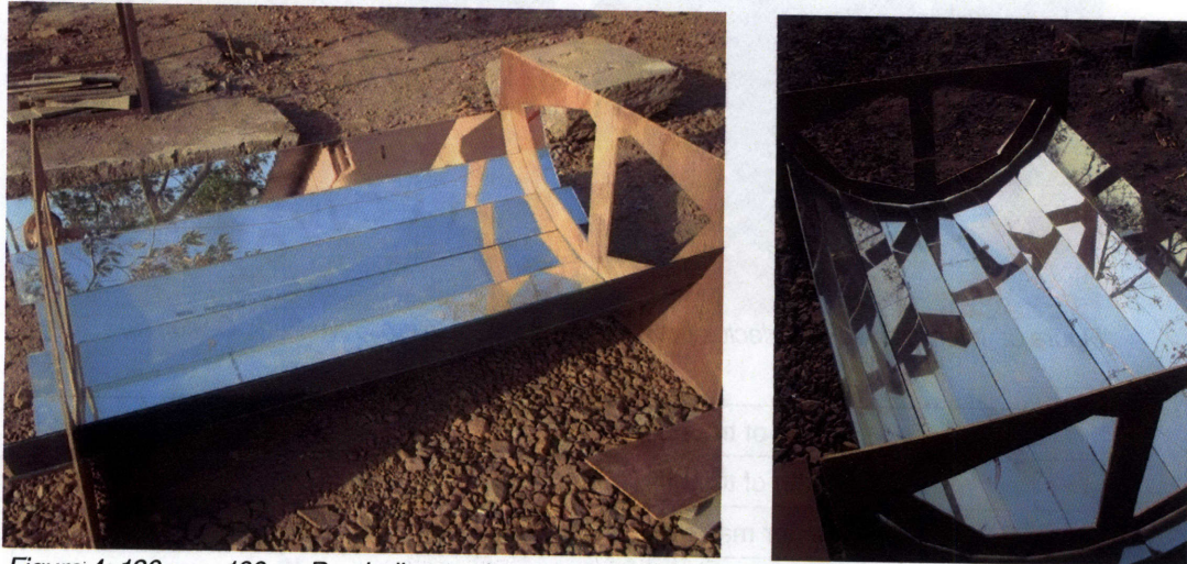
Figure 4: 180cm x 100cm Parabolic trough made from mirrored glass slats (Pabal, India)
