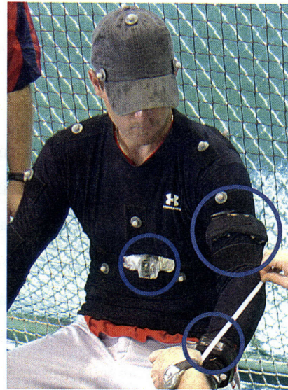
(b) Sensors being secured to the body of an athlete with straps and athletic tape.
