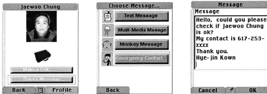
Figure 5.1(a) Detailed contact information, (b) Emergency Contact button, (c) Automatically composed message
