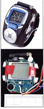
Figure 27: BellSouth™ FW13ZHS radio On the bunny side, a wristwatch sized transceiver, a BellSouth<sup>m</sup> FW13ZHS using the same spectrum, was stripped off its housing to minimize its footprint (Figure 27).
